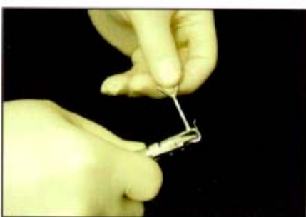
Figure 21. Torquing Upper Elbow
